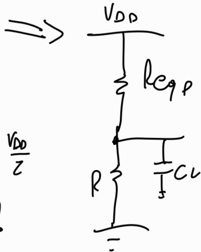
$$V_{out} = V_{DD} \cdot \frac{R}{R + R_{eqp}} = 2,3 \text{ V}$$
