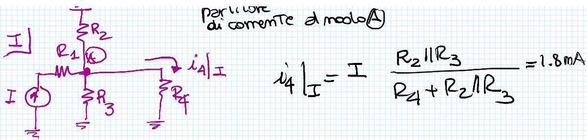
$$i_4 = i_4 |_{V_{dd}} + i_4 |_I \approx 1.8 \text{ mA}$$
