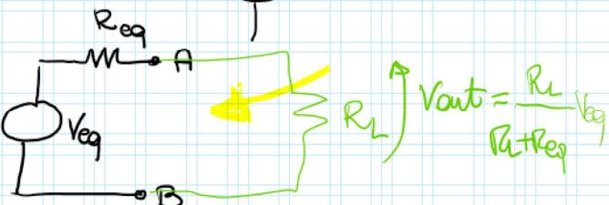
$$V_{out} = \frac{R_L}{R_{eq} + R_L} V_{eq}$$
