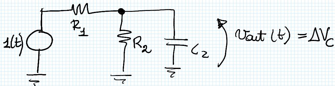
$$\gamma = C_2 (R_1 || R_2)$$
