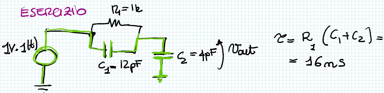
$$\gamma = R_2 (C_1 + C_2) = 16 \text{ ms}$$
