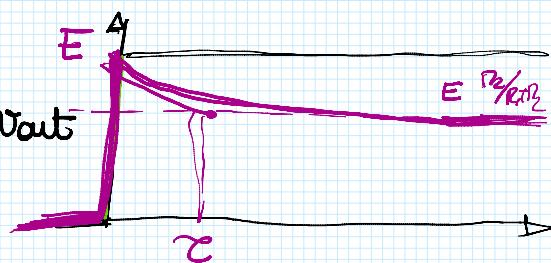
$$\gamma = C (R_1 \parallel R_2)$$
