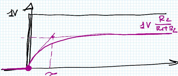
$$V_{out}(t \rightarrow \infty) = 1V \frac{R_2}{R_1 + R_2}$$
