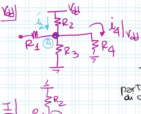
$$\begin{aligned} V_{dd} &= +5V & I &= 2mA \\ R_1 &= 400\Omega & R_4 &= 10\Omega \\ R_2 &= 500\Omega & R_3 &= 300\Omega \end{aligned}$$
