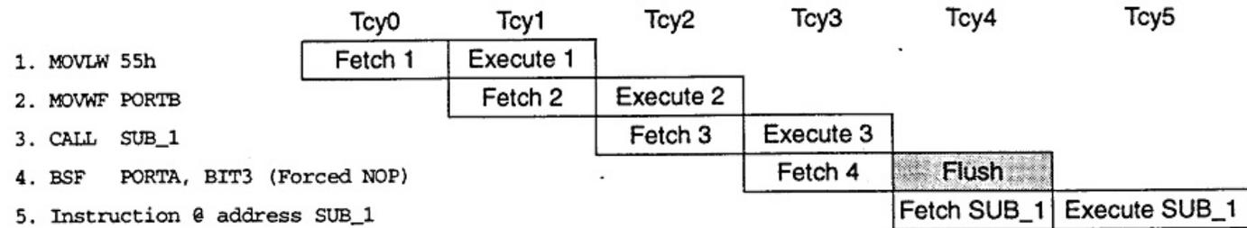
All instructions are single cycle, except for any program branches. These take two cycles since the fetch instruction is "flushed" from the pipeline while the new instruction is being fetched and then executed.
