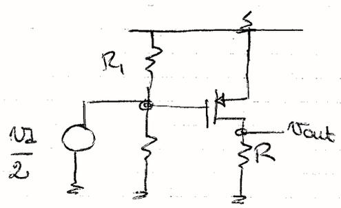
$$V_{out} = -g_m R \frac{V_1}{2}$$
