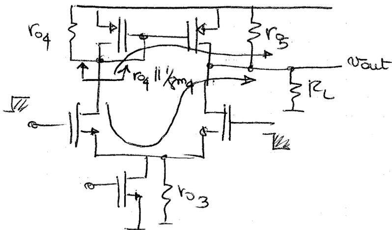
$$v_{out} = (r_{o5} \parallel R_L) \left[ g_{m1} \frac{v_d}{2} + g_{m1} \frac{v_d}{2} (r_{o4} \parallel \frac{1}{g_{m4}}) * g_{m5} \right]$$
