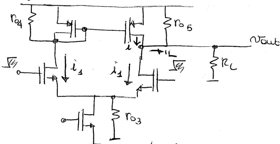
$$i = v_{CM} \frac{g_{m1} (r_{o4} \parallel \frac{1}{g_{m4}})}{1 + g_{m1} 2r_{o3}} * g_{m5} = \frac{g_{m1}}{1 + g_{m1} 2r_{o3}} \left[ \frac{r_{o4} \frac{g_{m5}}{g_{m4}}}{r_{o4} + \frac{1}{g_{m4}}} \right]$$
