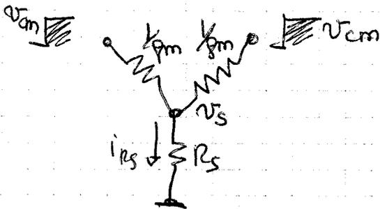
$$v_s = 2 \frac{\frac{1}{g_m} \parallel R_s}{\frac{1}{g_m} + \frac{1}{g_m} \parallel R_s} v_{cm} = \frac{2 R_s}{\frac{1}{g_m} + 2 R_s} v_{cm}$$
