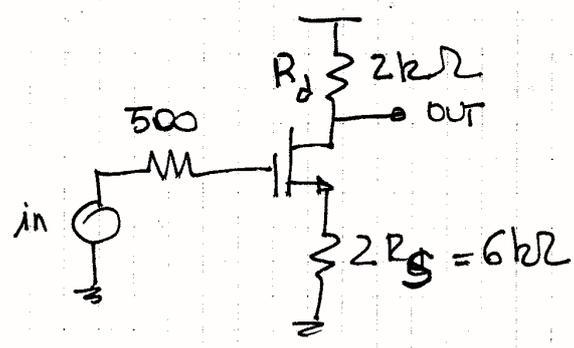
$$G_{CM} = -\frac{R_d}{\frac{1}{g_m} + 2R_s} = -\frac{R_d}{2R_s} = -0.333$$
