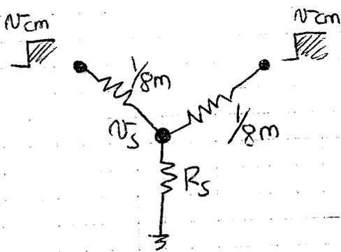
$$V_S = \frac{\frac{1}{g_m} \parallel R_S}{\frac{1}{g_m} + \frac{1}{g_m} \parallel R_S} N_{cm} + \frac{\frac{1}{g_m} \parallel R_S}{\frac{1}{g_m} + \frac{1}{g_m} \parallel R_S} N_{cm} = \frac{2R_S}{2R_S + \frac{1}{g_m}} N_{cm}$$
