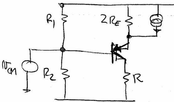
$$R_{cm} = \left[ (R_1 \parallel R_2) \parallel (r_{\pi} + 2\beta R_E) \right] \frac{1}{2}$$
