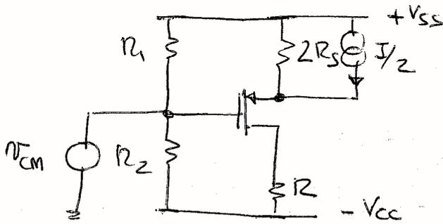
$$R_{cm} = \frac{1}{2}(R_1 \parallel R_2) = 25 \text{ k}\Omega$$
