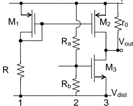
$$v_{out,1} = -v_{dist} \frac{r_0}{R + \frac{1}{g_{m,1}}}$$
