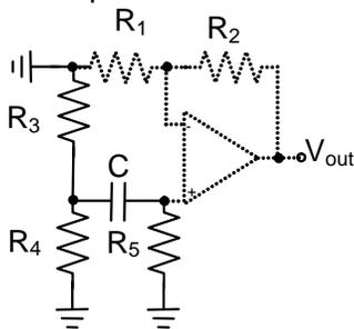
$$\tau_C = C[(R_4 // R_3) + R_5] = 1.33 \mu s$$
