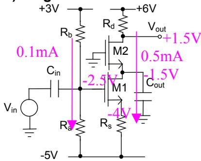
$$i_{d1} = i_{d2} = \frac{v_{in}}{\frac{1}{g_{m,1}} + R_s}$$
