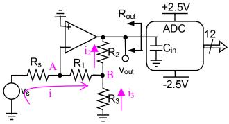
$R_{I}$ =1k $\Omega$   $R_{2}$ =100k $\Omega$   $R_{3}$ =1k $\Omega$   $R_{s}$ =1k $\Omega$   $C_{in}$ =15pF  $A_{0}$ =75dB
