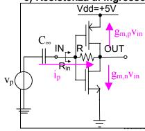
$$R_{in} = \frac{v_p}{i_p} = \frac{v_p}{2g_m v_p} = \frac{1}{2g_m} = \frac{1}{6mS} = 167\Omega$$
