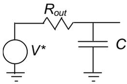
$$V^* = \frac{V_{out,a}|_{ideale}}{1 - \frac{1}{G_{loop}(0)}}$$
