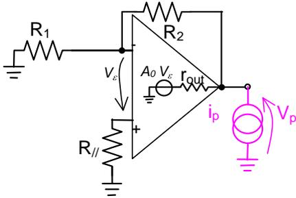
$$R_{out} = \left[ \frac{R_{out}|_0}{1 - G_{loop}^*(0)} \right]$$
