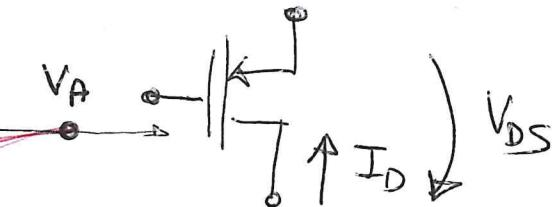
$$I_{D_{sat}} = k_p (V_{GS} - V_{TP})^2 (1 + 2V_{DS})$$
