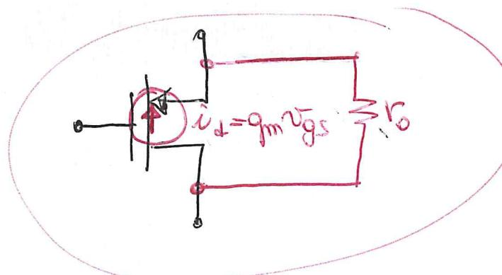
$$\frac{\partial I_{D_{sat}}}{\partial V_{DS}} = \frac{\partial [k_p (V_{GS} - V_{TP})^2 (1 + 2V_{DS})]}{\partial V_{DS}}$$
