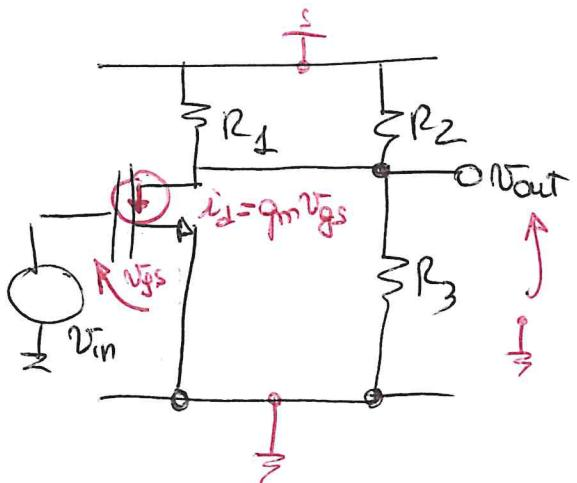
$$V_{out} = -i_d (R_1 \parallel R_2 \parallel R_3) = -g_m V_{gs} (R_1 \parallel R_2 \parallel R_3) = -g_m V_{in} (R_1 \parallel R_2 \parallel R_3)$$
