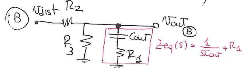
$$\text{polo } \omega_p = \text{Cout} (R_1 + R_2 \parallel R_3) \Rightarrow f_p = 2.7 \text{ Hz}$$
