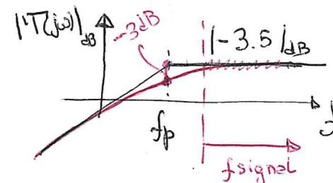
$$|T(s)| \triangleq \frac{V_{out}(s)}{V_{in}(s)}$$
