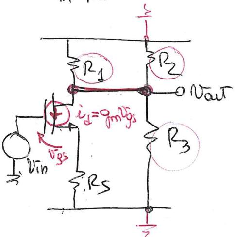
$$V_{out} = -i_d (R_1 \parallel R_2 \parallel R_3)$$
