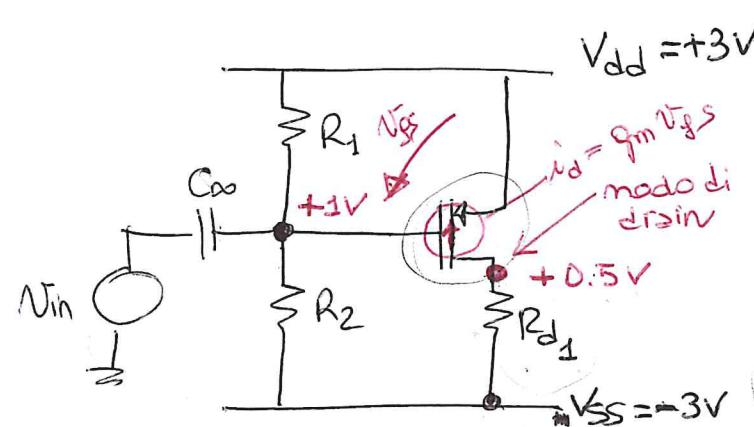
$$V_{D\text{drain}} = -i_d R_{D1} = -gm V_{in} R_{D1}$$
